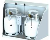
a = GasStop b = Hose (high-pressure) c = Bulkhead pressure regulator with automatic/manual changeover device
