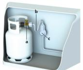
a = GasStop b = Hose (high-pressure) c = Bulkhead pressure regulator
